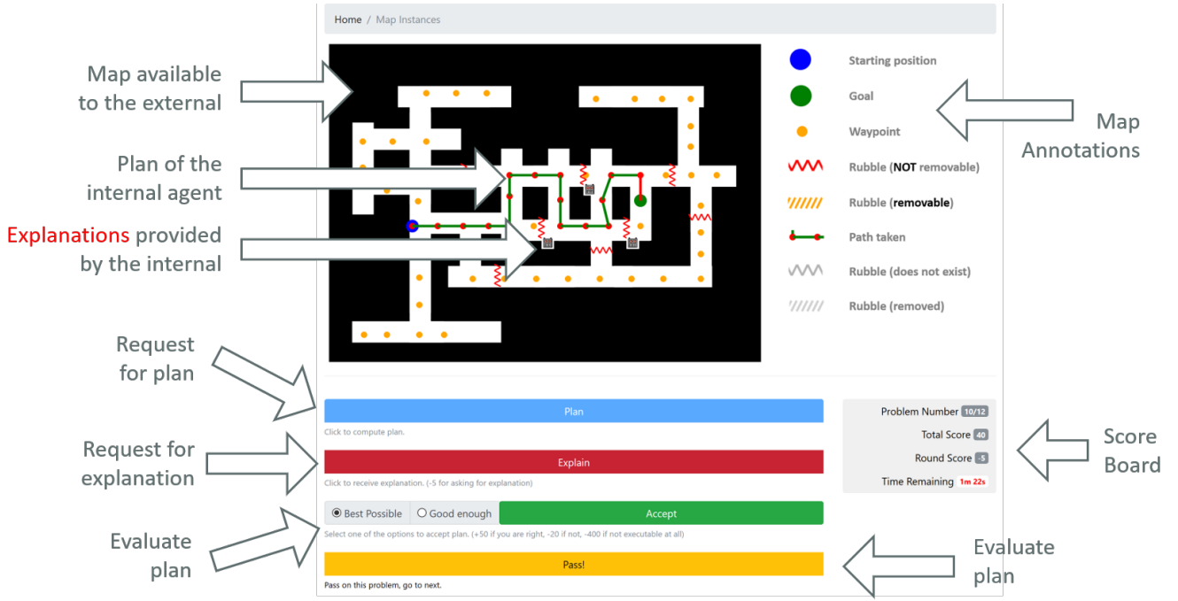
Figure 7: Interface for Study-2 where participants assumed the role of the external commander and evaluated plans provided by the internal robot. They could request for plans and explanations to those plans (e.g. if not satisfied with it) and rate those plans as optimal or suboptimal based on that explanation. If still unsatisfied with the plan even after the explanation they could chose to pass and move on to the next problem.
