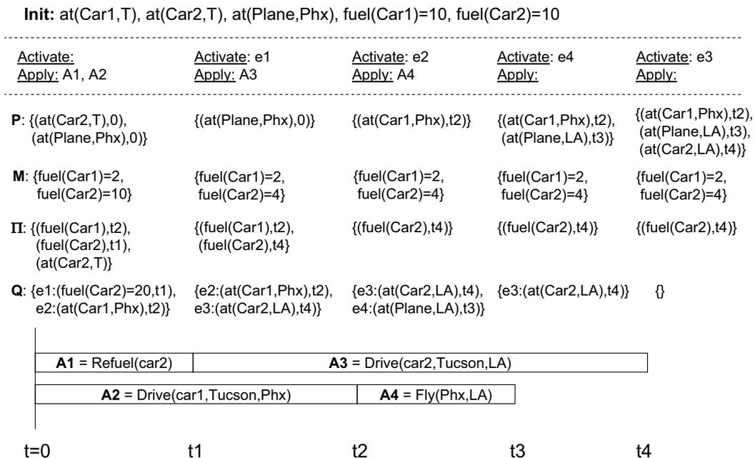
Figure 8. An example showing how different datastructures representing the search state  $S = (P, M, \Pi, Q)$  change as we advance the time stamp, apply actions and activate events. The top row shows the initial state. The second row shows the events and actions that are activated and executed at each given time point. The lower rows show how the search state  $S = (P, M, \Pi, Q)$  changes due to action application. Finally, we show graphically the durative actions in this plan.
