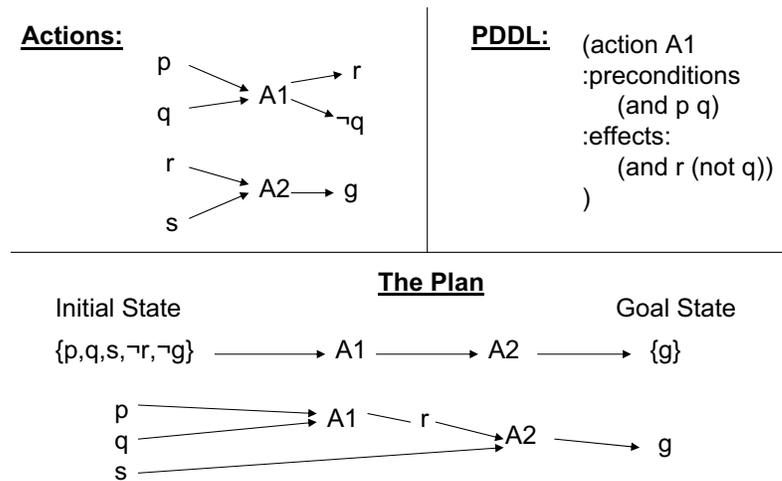
Figure 3. Example of plan in STRIPS representation.
