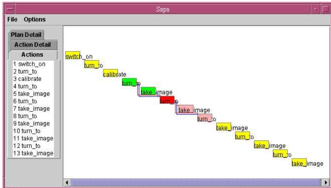
Figure 15. Screen shots of *Sapa*'s GUI: Gantt chart showing different logical relations between a given action and other actions in the plan.
