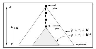
Figure 2: Successful replay reduces the size of the search. However it entails the additional cost,  $\rho$ , of retrieving a trace from the library, as well as the cost,  $\eta$ , of validating each of the decisions in the trace. When replay fails performance may be worse than in from-scratch planning.
