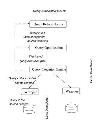
Figure 1.1 Prototypical architecture of a data integration system
