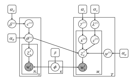
Figure 3.2: Graph Model of Et-LDA. S(T) Is a Set of Paragraphs (Tweets).  $Z_s(Z_t)$  Is the Topic for Paragraph s (Tweet t), Which Can Be Drawn Either from Topic Mixture  $\theta^{(s)}$  of the Event or Topic Mixture  $\psi^{(t)}$  of the Tweets Corpus. Shaded Variables  $W_s^i$ and  $W_t^i$  Are the *i*th Word in s and t and Are Observed in the Dataset.
