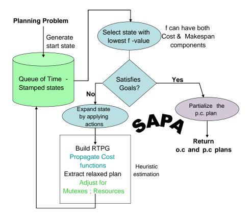
Figure 1. Architecture of Sapa
