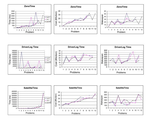
Figure 17. Comparison of the different lookahead options in the competition domains. These experiments were run on a Pentium III-750 WindowsXP machine with 256MB of RAM. The time cutoff is 600 seconds.
