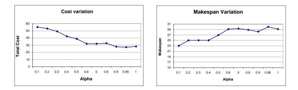
Figure 16. Cost and makespan variations according to different weights given to them in the objective function. Each point in the graph corresponds to an average value over 20 problems.
