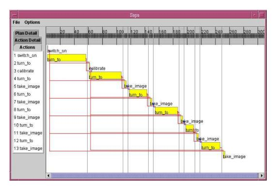
Figure 14. Screen shot of *Sapa*'s GUI: PERT chart showing the actions' starting times and the precedence orderings between them.
