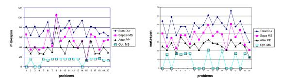
(a) With *drive inter-city* action.(b) Without *drive inter-city* action.Figure 27. Compare different makespan values for random generated temporal logistics problems
